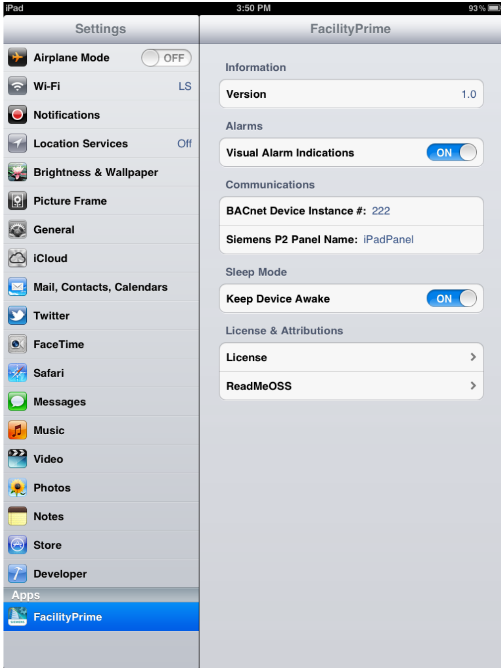
Figure 9: Settings for an iPad's Facility Prime Application.
